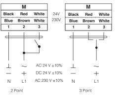
A Connect via safety isolating transformer
