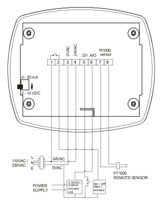
Note : If Emergency IP [D/I] not used then add link between terminal No 5 & 3.
