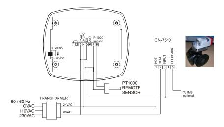
E]WIRING DIAGRAM T2798I2000 WITH VC-7934
