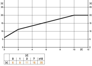
[d] = Power failure in days [s] = Pre-charging time in seconds
