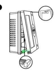
Surface mounting in a 60mm wall box. Make sure the back cover is in the appropriate position (according to the arrow on it) Fit the front part of the casing to the top edge and make sure the pins are properly positioned. Push the front of the casing until you hear positive click.
