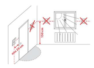
Devices must be mounted on clean, dry indoor place without direct airflow from a heating / cooling device, and not be exposed to dripping or splashing
