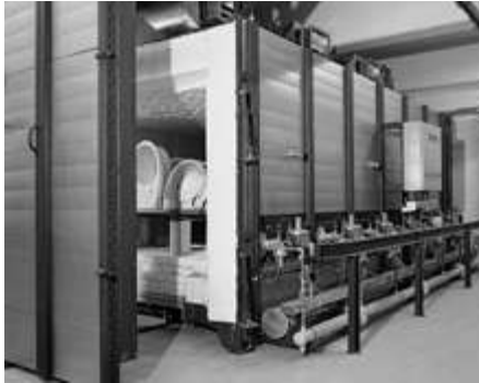
Intermittent shuttle kiln in the ceramics industry
