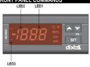
SET: in normal mode is not used. In programming mode is used to select parameters or confirm a value.
