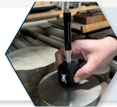
This version of the device can connect to NOVOTEST Lab. Combined with a smartphone, it turns into a small portable multifunctional device for measuring, logging and sharing hardness testing results.
