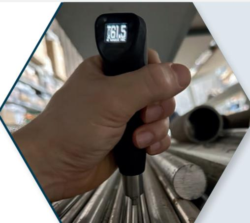
The contrast display allows users to do measurements not only in NOVOTEST Lab, but also without a smartphone. This makes hardness testing quick and easy. The ergonomic design ensures a comfortable grip, preventing slipping, and is suitable for both right- and left-handed users.
