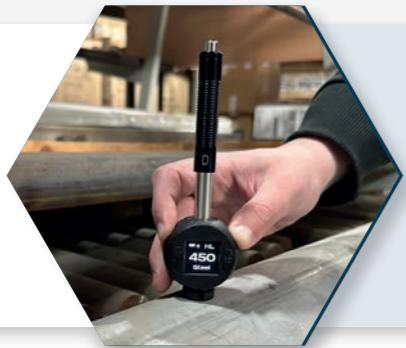
This method is usually used for large products. Its advantages include the application for materials with a coarse-grained structure, non-ferrous metals, low requirements for the quality of the test object surface, as well as ease of use.
